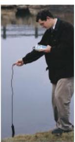
One meter does it all—measure pH, conductivity and temperature without switching meters or probes! Switch between conductivity and pH with a button press. Meters read pH from 0 to 14 pH, conductivity over four ranges up to 19.99 mS, and temperature in °C. Three-point pH calibration with auto-buffer recognition and four-point conductivity calibration provide high accuracy.
